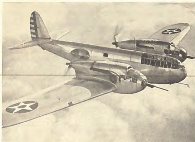
BELL XFM-1 tomoloret, tung Jager, hvis Motorer driver to Trykpropeller.
