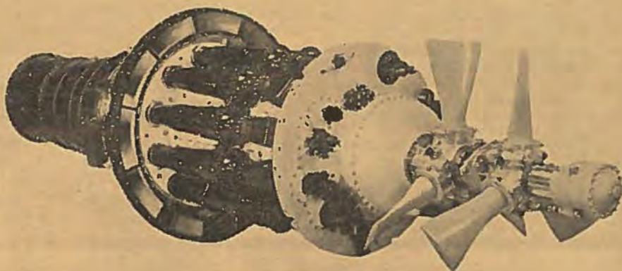
Englands kraftigste propel-turboreaktor, Armstrong-Siddeley Python I yder 3670 hk plus 521 hk trykkraft. Diameter 122 cm.
