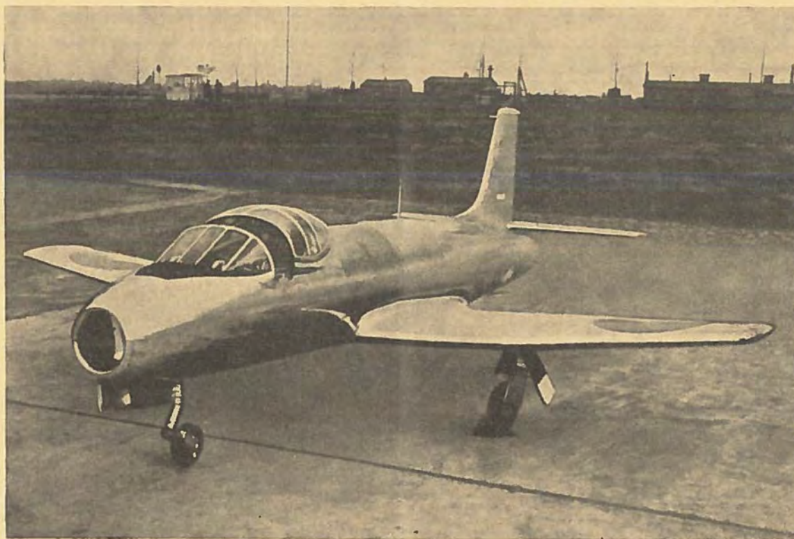
THE FOKKER S. 14, SIDE-BY-SIDE JET TRAINER powered by the Rolls-Royce „Derwent“ turbo-jet engine
