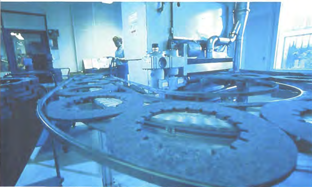
Kulfiber bremseskiver under renovering.
