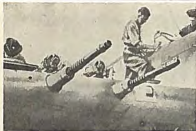
Fig. 5. 20 mm MK i Vinge. (Oerlikon i Hawker Hurricane).
