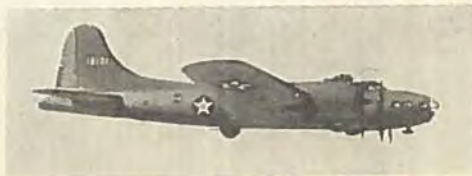
Fig. 17. 4-mot. Bomber: Boeing Fortress. 12 Stk. 12.7 mm. M.G. 7 - 7.6 - -
