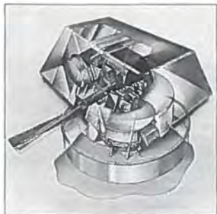
The stealth designed cupola is ready for the coming generation of SES ships.
