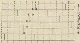
FIG. 99A.—Shift of Butts in Shell Plating. 5 frame spaces. Period 2 2 2 or 3 3 3. (4 passing strakes.)
