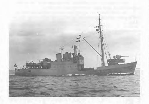
TYPE: Coastal Minelayer LANGELAND-class NAME: NUMBER: LAID DOWN: COMPLETED: LANGELAND N.42 1950 1951 Displacement: 330 Length ft.: 134 24 Beam ft.: Draught ft.: 7 Engine: 2 diesel engines each of 200 BHP
